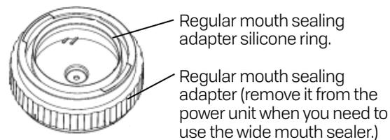
Prior to use, check that the silicone ring is installed properly. This will ensure correct function of the sealer.
